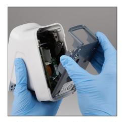
6. After the base has dried, reattach it to the device and ensure it is locked into place.
