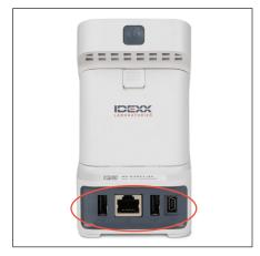
Power off the device and disconnect the power and/or Ethernet cord.
