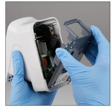
3. Remove the base from the device.
