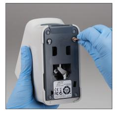
2. On the bottom of a powered-off device, use a flat-tip screw driver or coin to turn the 2 silver fasteners counterclockwise a quarter turn.
